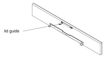
Step 4: Install the hinge receiver plates 17" on center of back fixed portion of the lid.
